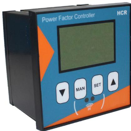
Automatic power factor controllers with microprocessor designed for signal processing of strongly distorted waveform to ensure accurate control of the electrical parameters of the plant. All measurements are made starting from the analysis of the waveform using FFT (Fast Fourier Transform) algorithm in floating point to ensure the maximum precision.
