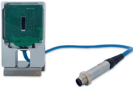
The Solarimeter with serial output is a high-tech electronic device designed to accurately measure the solar radiation and make it available to the user in the best way suitable for its applications.
