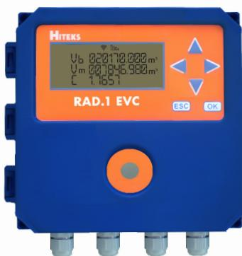
**RAD.1 EVC** is a gas volume corrector that provides a powerful solution for commercial gas measurement purposes. The device is designed to convert the volume of gas measured under operating conditions to volume under base conditions; it measures gas temperature and pressure in compliance with MID standards.
