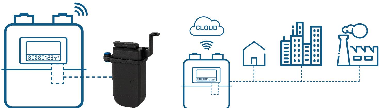
The **HYSPI** is an AMR module mounted on existing mechanical (diaphragm) gas meters or connected to the impulse output of commercial meters and volume correctors using cable connectors.
